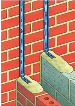
Creates an easy way to tie in new walls to existing brickwork without cutting out
